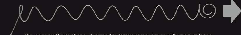
The unique aSpiral shape, designed to form a strong frame with random loops by having 1:1 ratio between coil diameter and pitch (≥ 7 mm coil)
