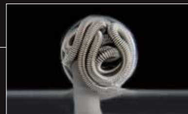
2-4ES (φ2mm x 4cm) tightly packed in a 2 mm aneurysmal model.
